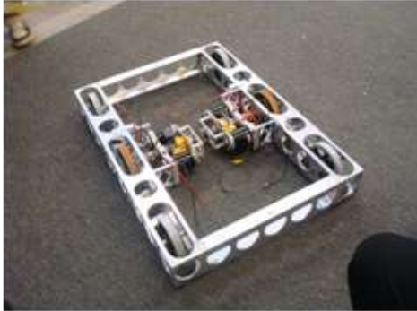
Figure 1.2-4 This is the six wheel drive base that we constructed during the 2008 off season.
